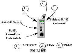
The PM-RJ45 will support 10BASE-T unshielded twisted pair wiring (UTP) environments with maximum segment distances up to 100m (325 ft.), or shielded twisted pair wiring (STP) of 150m (500 ft.). This module is designed with internal transceiver functionality. The PM-RJ45 has ACTIVITY, LINK and SPEED LEDs.
